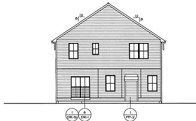
3 A-2c REAR ELEVATION SCALE: 1/8" = 1'-0" ELEVATION K "ELK" ELEVATION L "ELL" SLIDING GLASS DOOR "DGT" GAS FIREPLACE FAMILY ROOM REAR "LGF"
