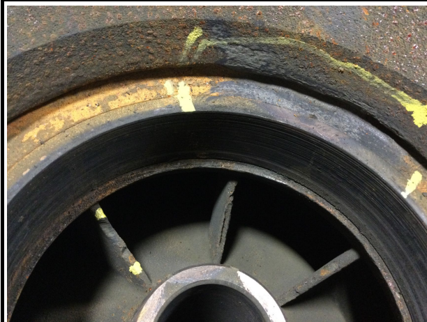
6. Cut adapter case due to motor seizure.
