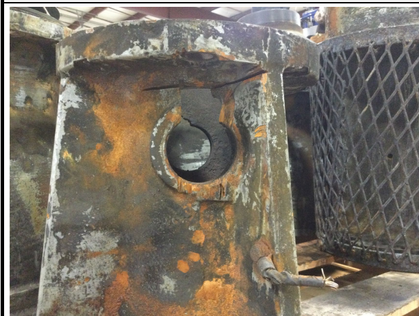
6. Cut adapter case due to motor seizure.
