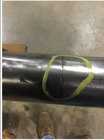
3. Bowl washed at wear ring critical area
