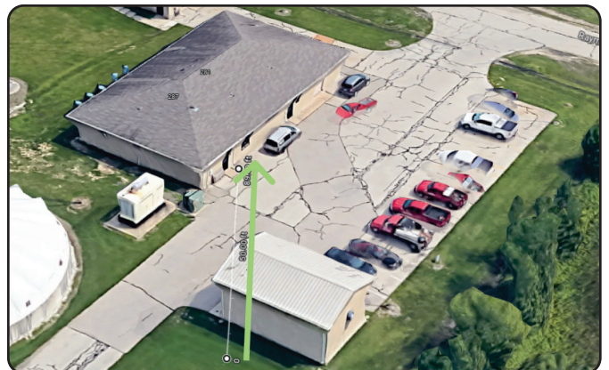
O'Carroll to bore new feed from grassy area to Wastewater Treatment Facility; we will trench to the failed pole lights and restore power to those, as well as the (3) roadway lights on that failed circuit
