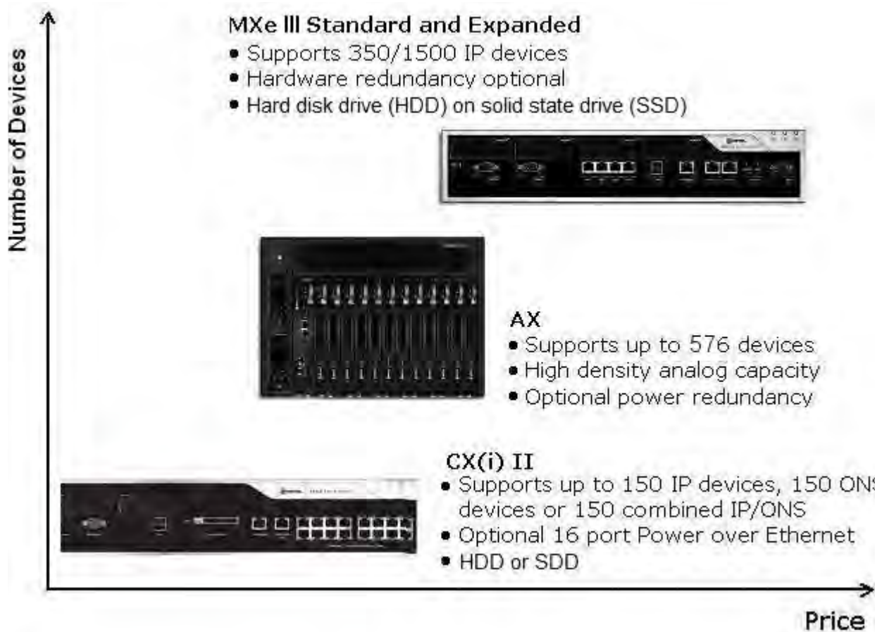
Figure 14: 3300 ICP Controllers — Scaling to Site Requirements
