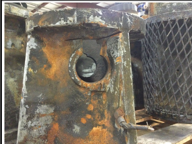
6. Cut adapter case due to motor seizure.
