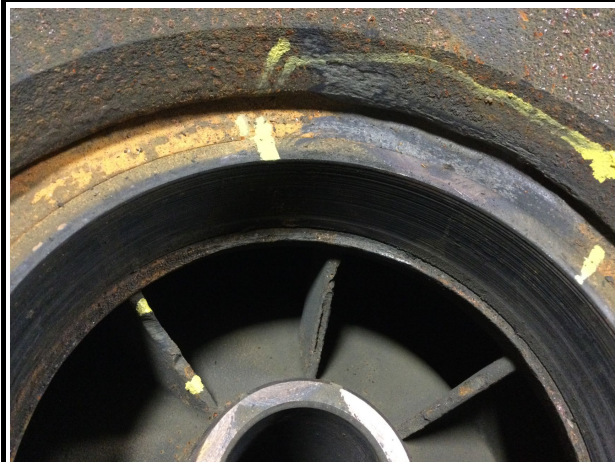
6. Cut adapter case due to motor seizure.
